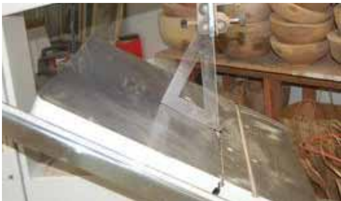
The bandsaw is set at the desired cutting angle
