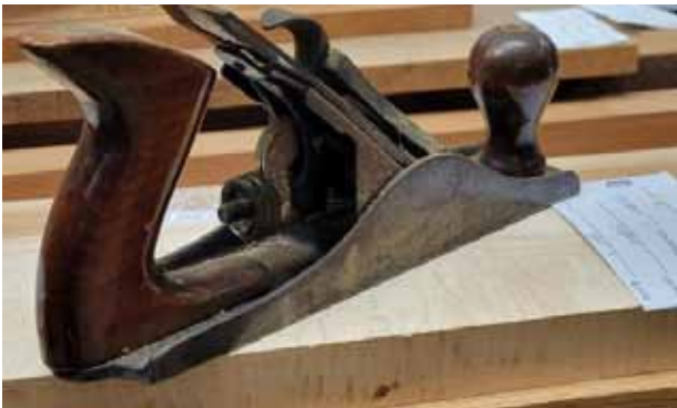
Plane with brass adjusting screw, high knob, and lateral adjuster
