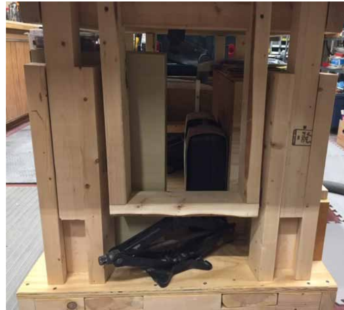
Scissors jack adjusts table height
