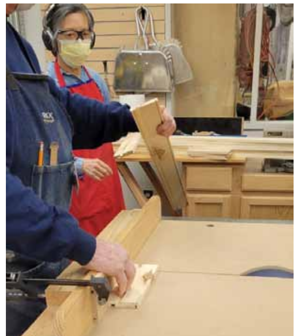
Stock with grooves cut for top and bottom panels
