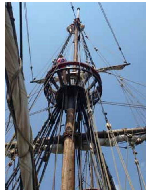
The stepped mast with its support shrouds and stays.
