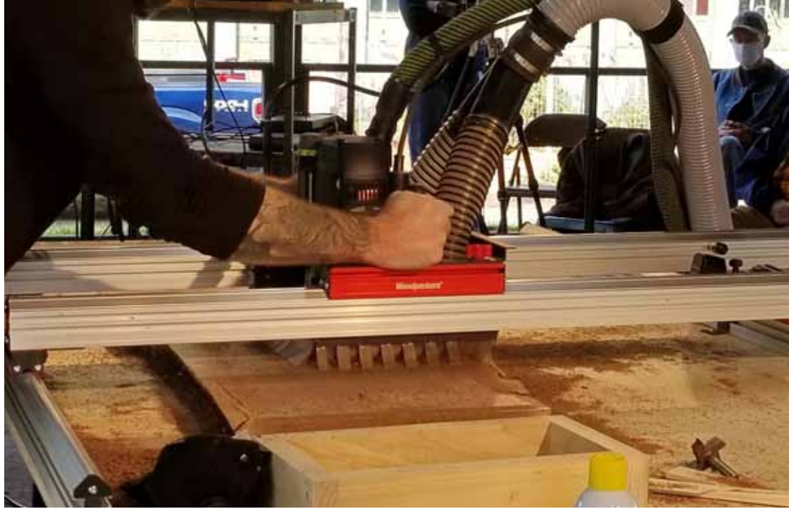
The slab flattening set up
