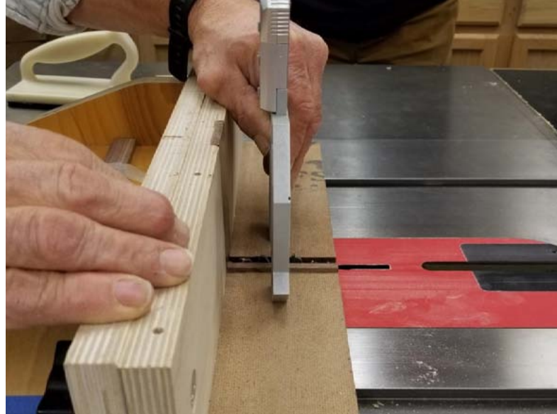
#3 Joe sets the 1/4" dado blade's height for cutting finger joints
