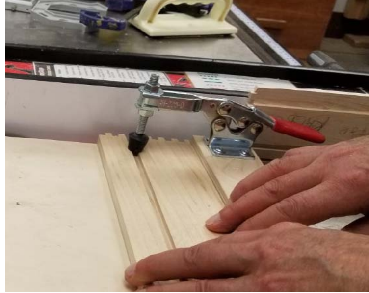
#9 Saw and new jig with clamp set to cut rabbets
