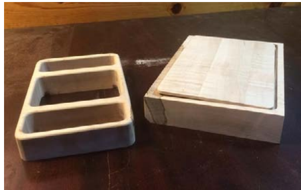
A small round over bit is used at the router table to ease the top edges of the insert and the inside of the box. The bottom is fitted. Normally I would chisel out the corners, but I was afraid of breakout on the short grain ends, so I rounded the insert corners on my stationary sander.
