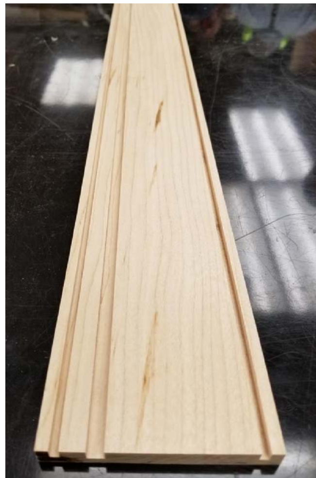
#1 Grooves are cut for top and bottom panels and lid
