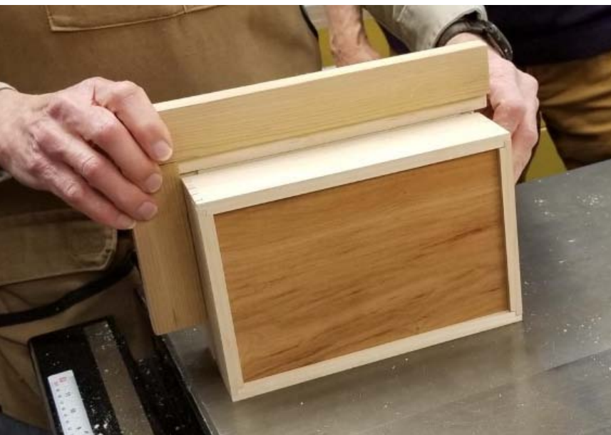
#12 Using the spacer for cutting the last two sides of the lid prevents movement
