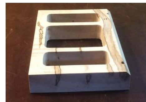
#2 Using an mdf template and plunge router with a bushing installed, rout the three inside openings.
