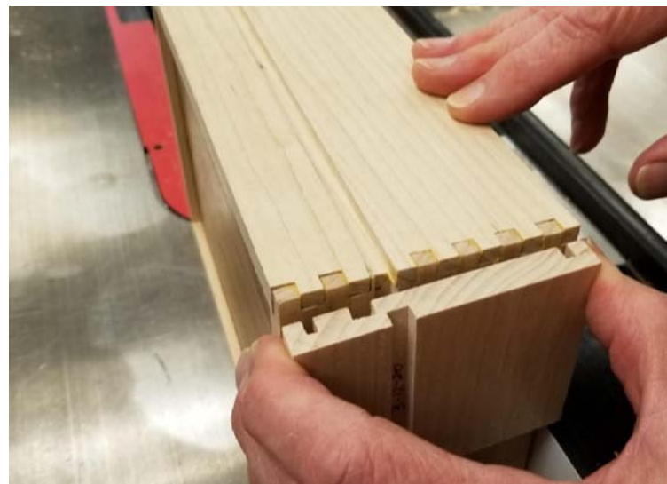
#11 Setting the fence to the box lid groove
