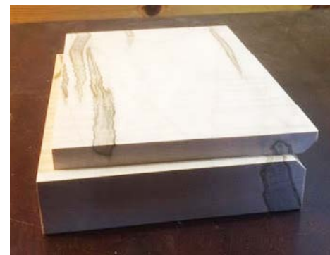
Bandsaw the 1/2 in thick top and bevel the edges where the barrel hinges go.
