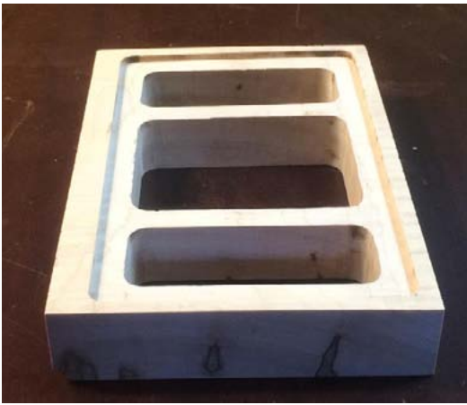
With another mdf template rout the recess for the bottom using a 1/2 in pattern bit.
