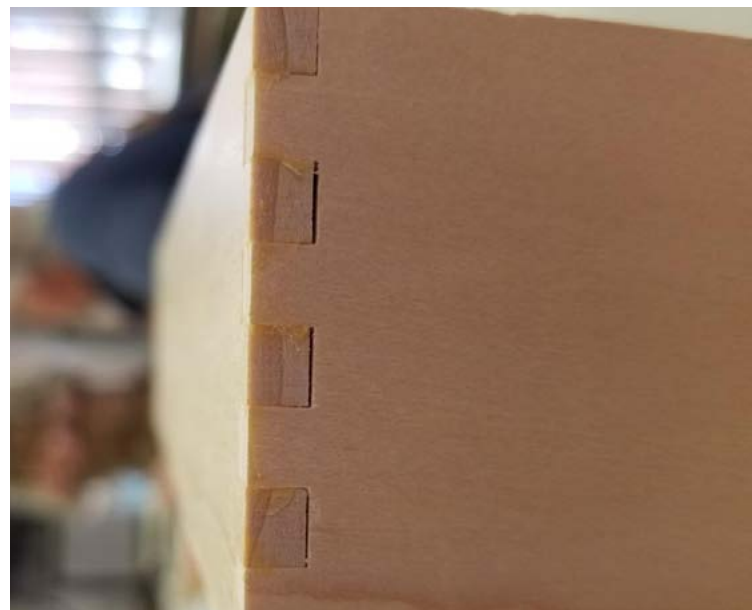
#13 Perfect finger joints made with the table saw and jigs
