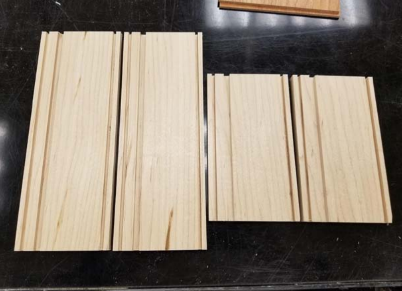
#2 Four sides are cut with the miter saw
