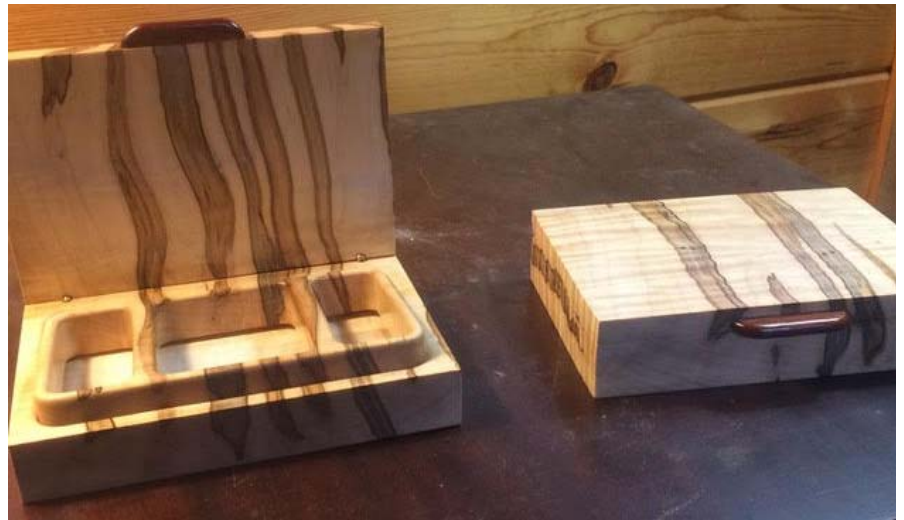
Almost done. Just a couple of more coats of Waterlox and a felt bottom will hopefully match the bloodwood handle. The insert is raised up a bit to show the matching figure.
