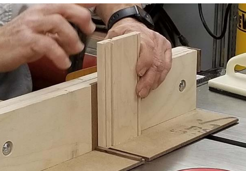
#6 The proper positioning and hold of short sides
