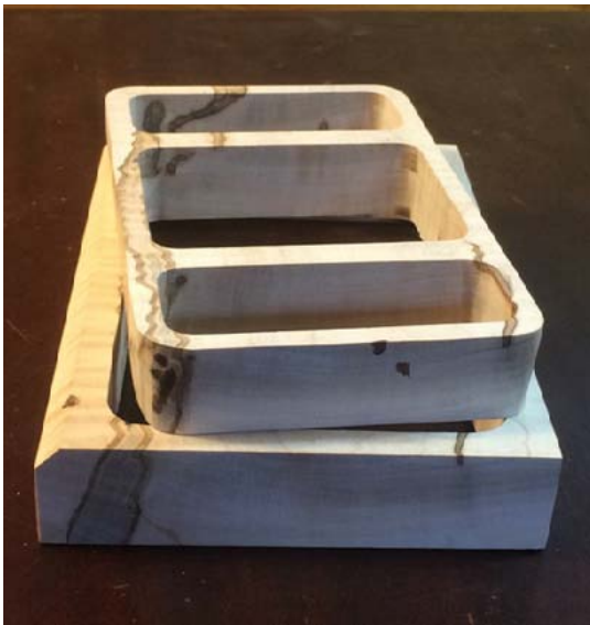
Scroll saw the insert away from the box. I used a #5 double reverse blade. Patience and a slow stroke and feed rate prevented burning in the 1 + in thick maple.
