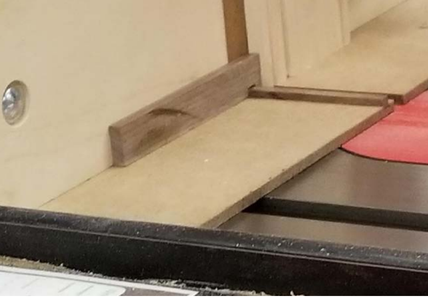
#8 A spacer is used for the first cut of the long sides
