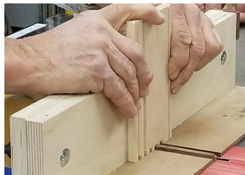
#7 The repetitive cut of fingers while moving the side toward the fence
