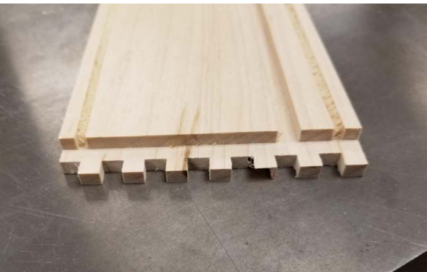
#10 Rabbets on all eight ends of four sides make a tight 90 degree fit
