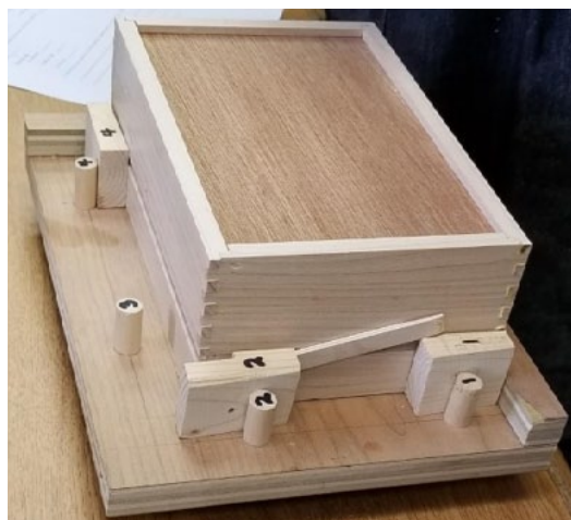
#10 Jig used to square up glued box
