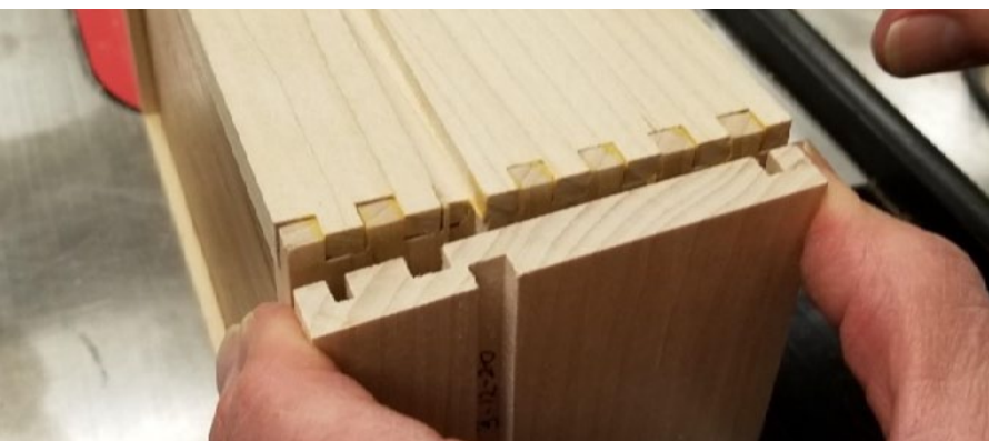
#12 Setting fence to box groove to cut off the top.
