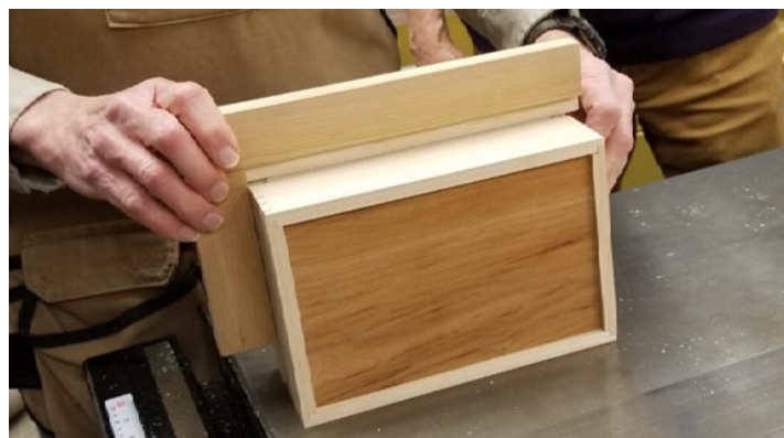
#13 Separates top from box to finish cuts without collapse
