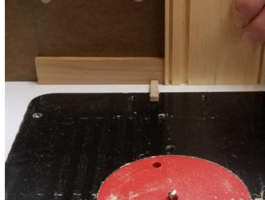
#6 Using a spacer for the first cut only, the longer sides' fingers are cut
