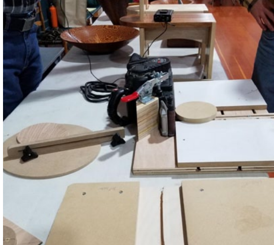
Jig can make and sand a variety of size disks
