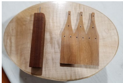
Cerruto's finger pattern and pin for box making
