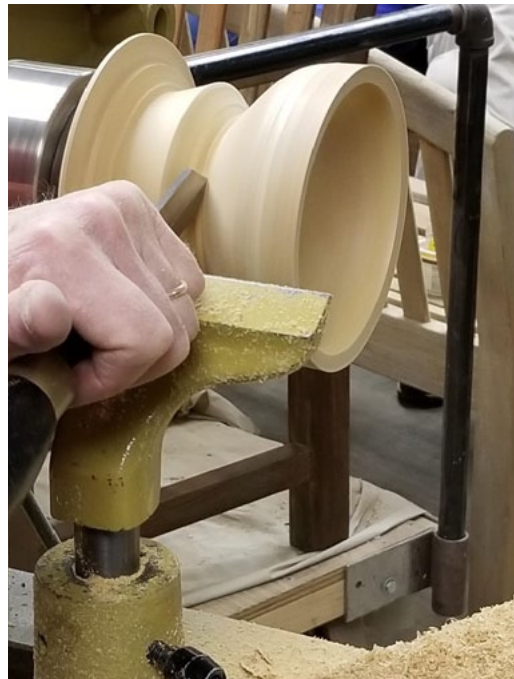
The parting to begins to separate the bowl from its base
