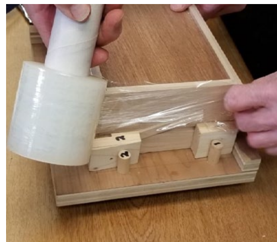
#11 Plastic wrap tight around box joints
