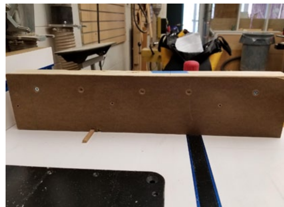
#3 The jig used to cut the fingers on the router
