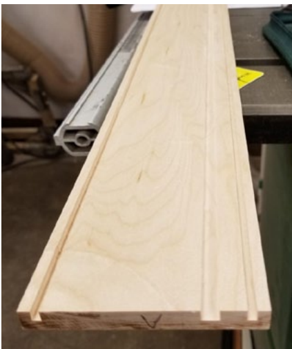
#1 Hard maple board 3\frac{7}{16} " x 34+ " with \frac{1}{4} " grooves for top and bottom
