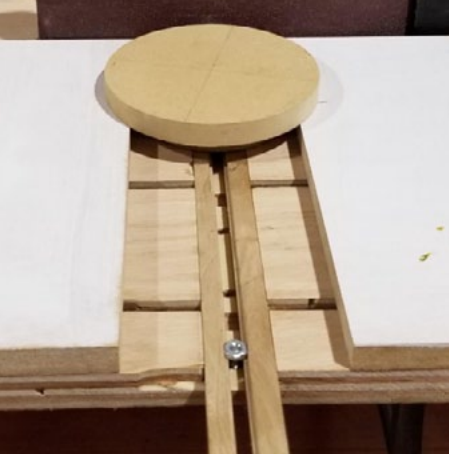
Andy Moss's bandsaw jig to make wooden CDs
