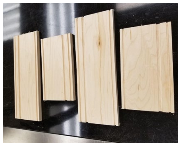
#2 Four sides are cut from board with miter saw: two 6" and two 9"
