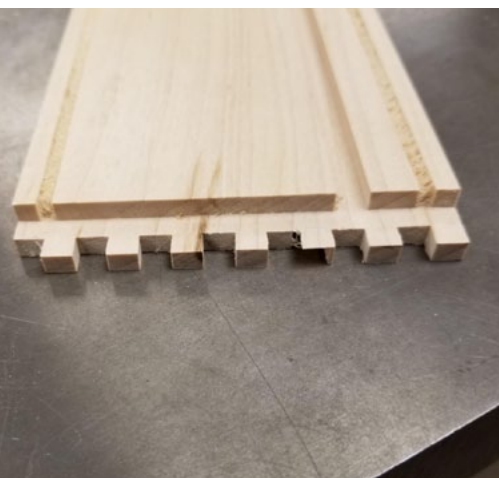
#9 Rabbets on all inside ends to make 90- degree fir to box corners
