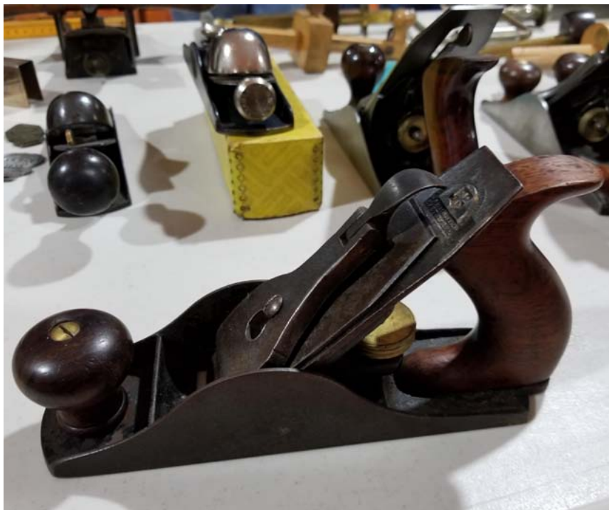
Leonard Bailey vertical post plane No. 3 (These planes were manufactured from 1861 until 1869)
