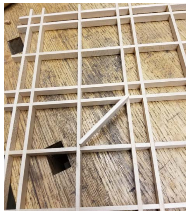
Step 1 is the cutting of diagonals
