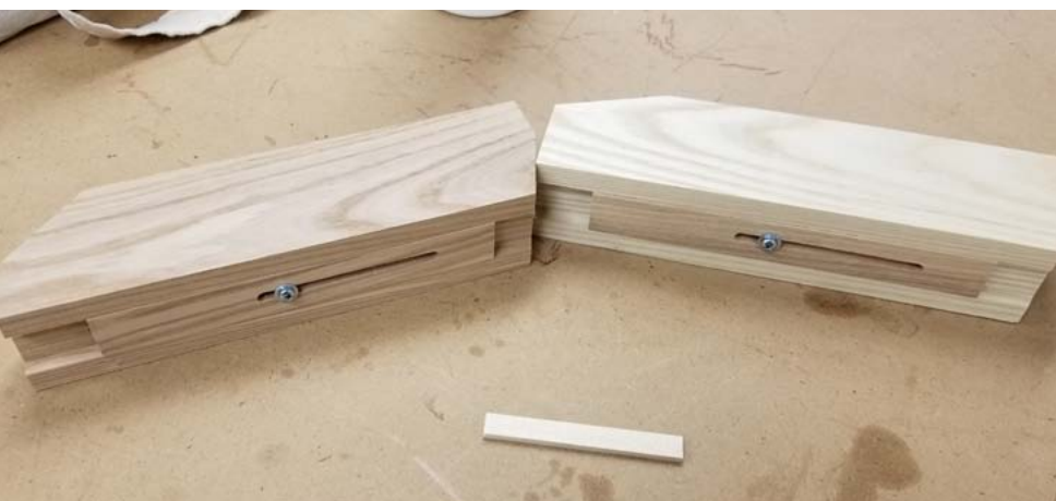
These custom-made jigs are used to pare exact angles
