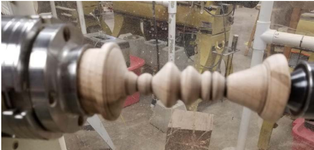
While turning, the chuck's tenon is cut from figure
