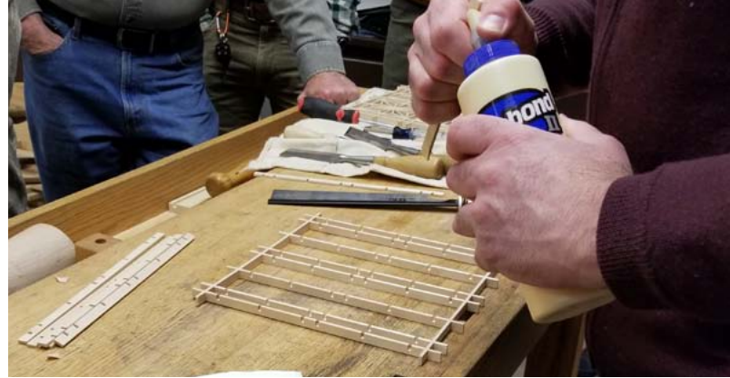
Matt assembles a frame (the only pieces to be glued)
