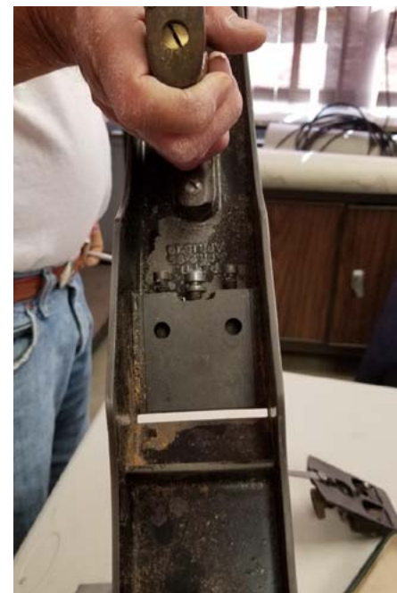
Bedrock has one point of iron contact with the frog
