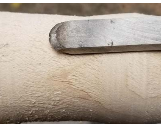
Round nose scraper smooths the wood
