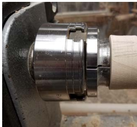
The three-jaw chuck grips the tenon
