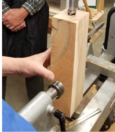
A mallet will drive the spur tailstock
