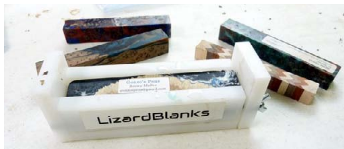
Cast materials employ resins and moulds
