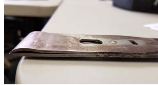
Chip breaker set very close to the iron's edge (1/32 ")
