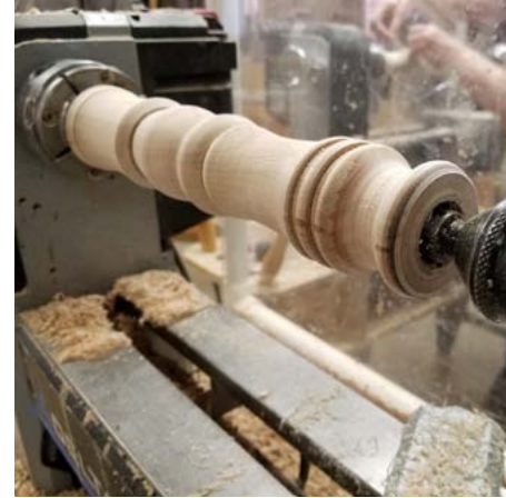
The tailstock spur at work
