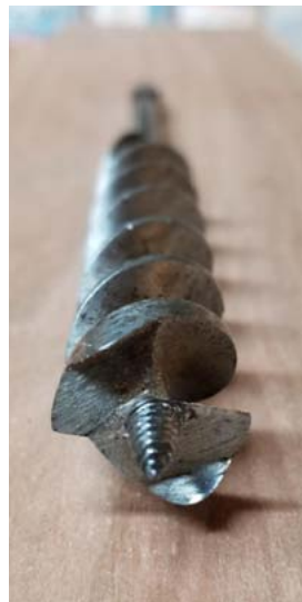
A bit's spurs and coarse lead screw
