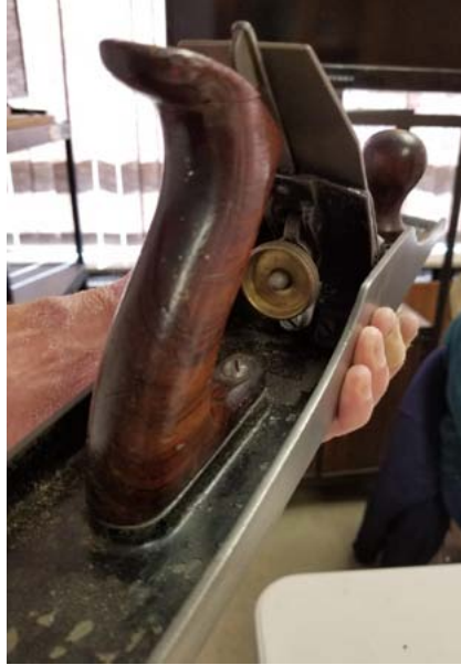
Bedrock planes have three screws to adjust the frog. This is a time saver for adjusting the frog.
