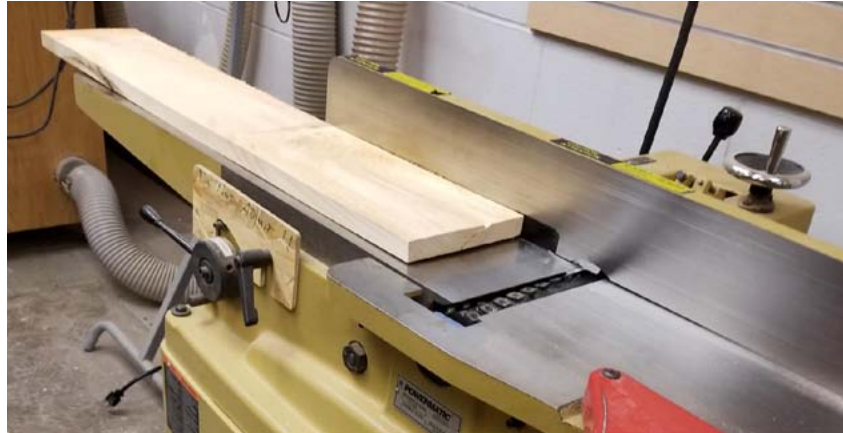
The infeed and outfeed tables on the jointer should be level to prevent snipe
