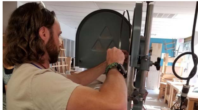
He removes the old blade without protective gloves!
