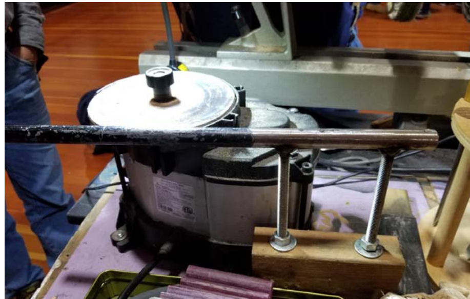
Ernie's custom-made tool rest for the Worksharp
