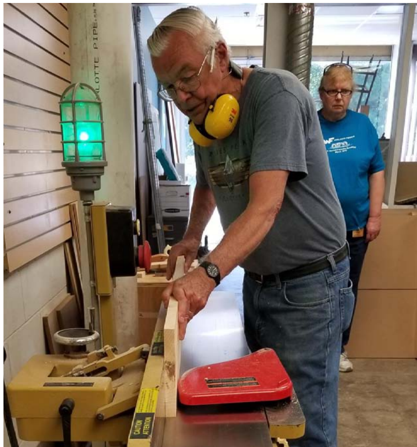
Charlie cuts a 90-degree edge to face with jointer
