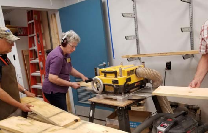
Feeding boards continuously end-to-end avoids snipe
