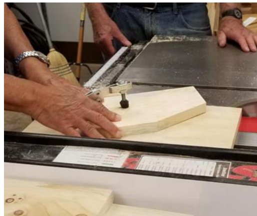
A jig holds the tote's side for an angle cut
