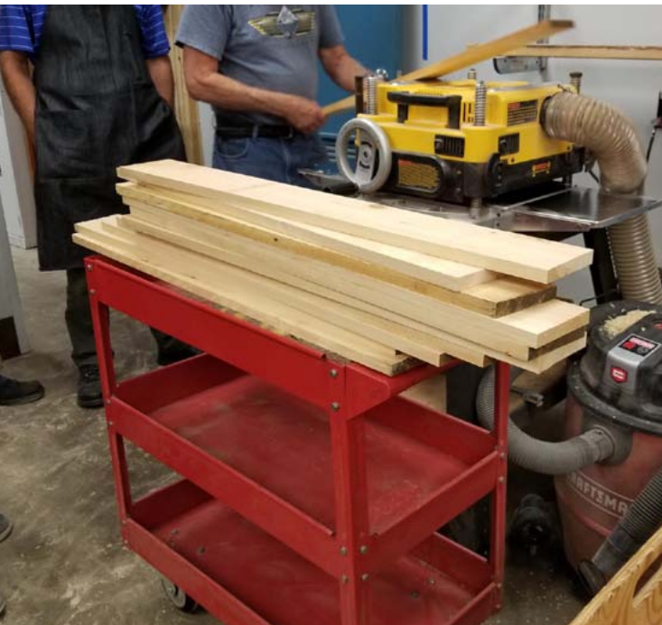
Totes' sides are planed to 1/2 inch thick
