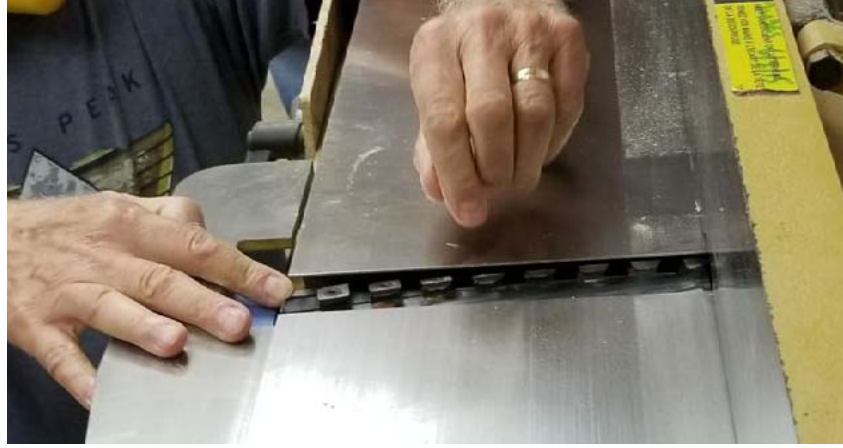
The jointer's cutter heads are helical
