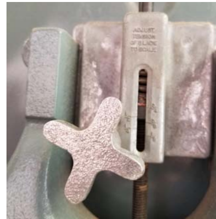
The tension gauge is not always accurate
