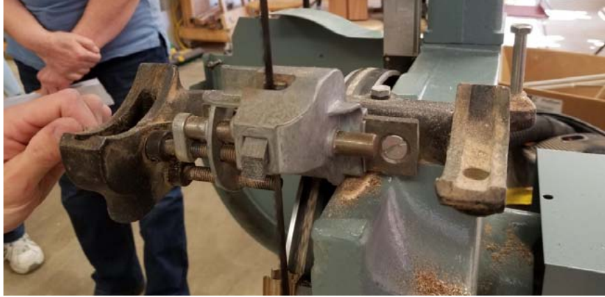
Cooling blocks set in lower blade guide
