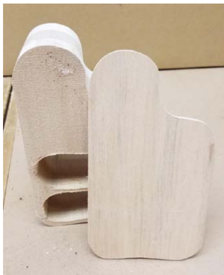
A box with the back sawn off ¼ inch thick
