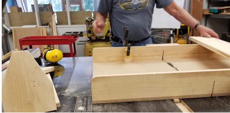
The table saw sled uses a stop block to make uniform cross cuts
