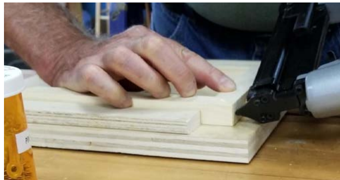
Jig ensures tight miter fit when tacked
