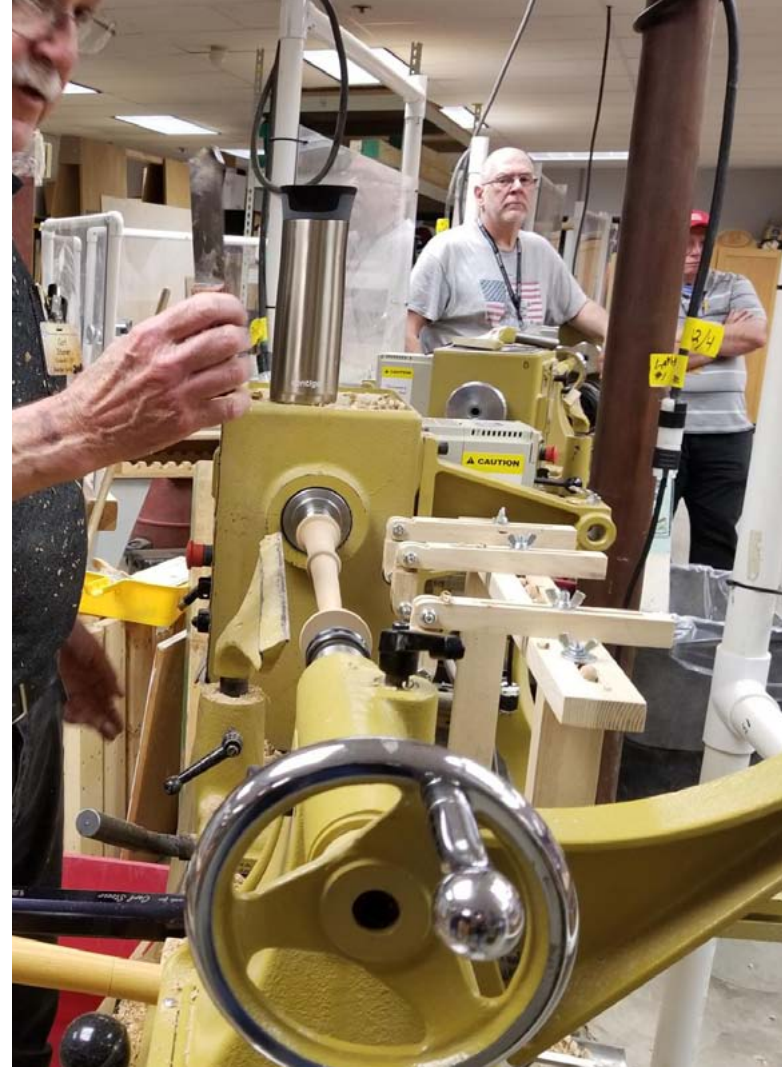
The jig's feelers drop down after the correct circumference is cut
