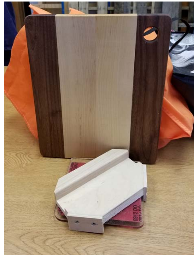
Hard maple and Sapele with Dave's cornering jig
