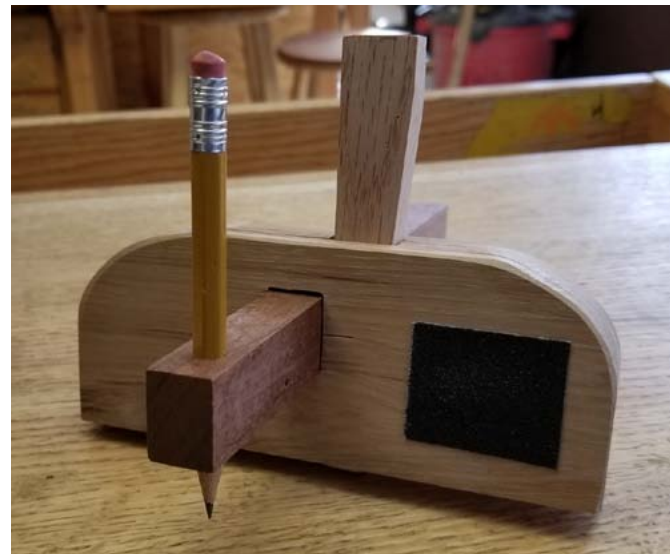
Model of Pencil Marking Gauge
