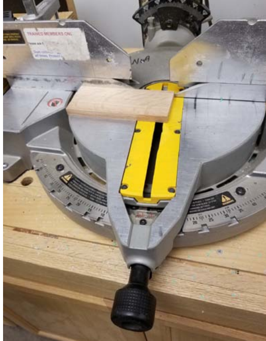
Miter saw cuts 15 degrees off one end of core
