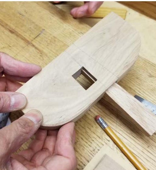
The wedge protrudes on one side of the hole about 1/8 inch
