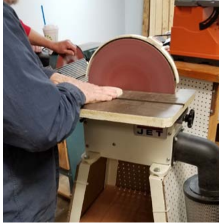
Bill sands a 4-degree bevel on the oval bottom
