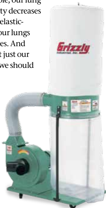
Whether the dust collector has a fabric or a canister filter on top, it can usually be equipped with a clear plastic disposable collection bag below; this offers the distinct advantage of allowing the woodturner to see at a glance when the bag is getting full.
