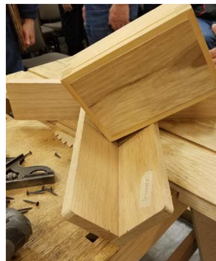
Goddard's jig for cutting box corners
