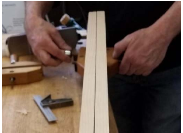
Plane two boards simultaneously
