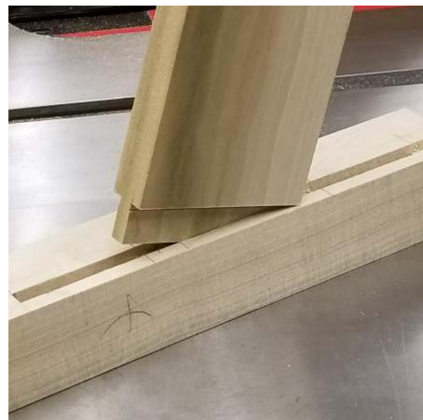
Resulting tight fit tenon
