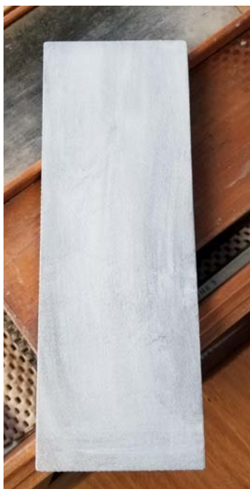
Diamond for flattening ceramic stones
