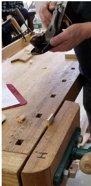
Use a wood chip to test an iron's uniform sharpness
