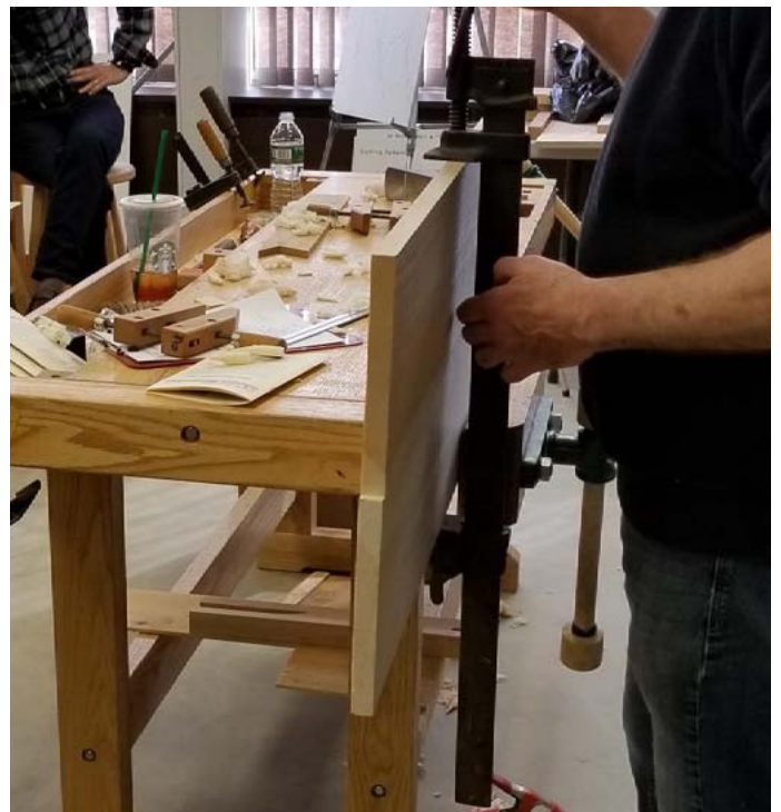
The spring joint for a tight, seamless glue up
