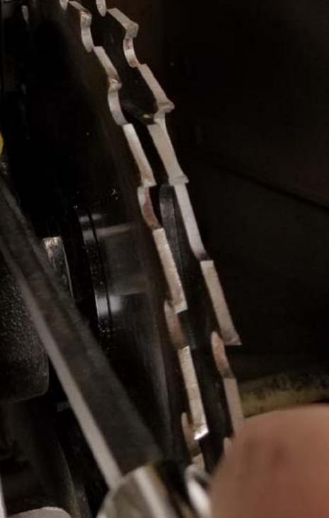
Two blades separated by a spacer to cut tenons
