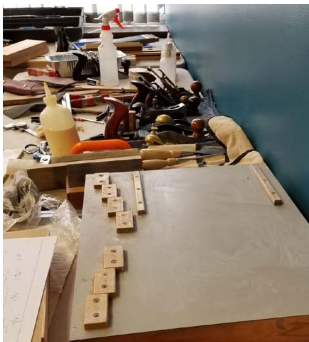
Bob's custom-made sharpening kit with jig
