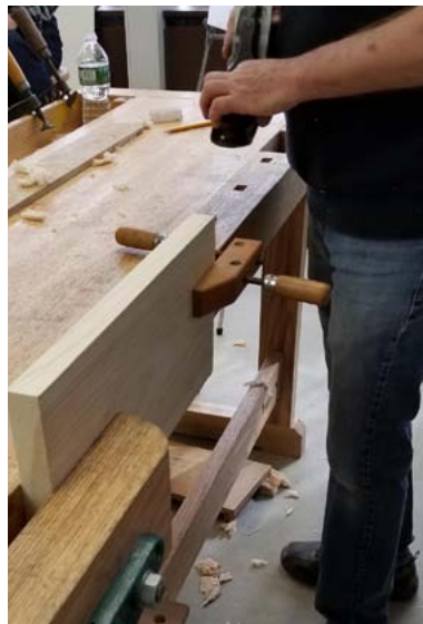
Use of clamp to keep a board stable in the vise
