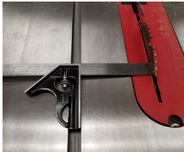
Precise Starrett measure of blade's distance from table track
