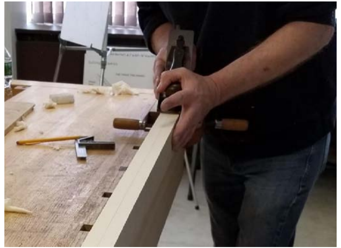
Make three passes in the middle third of boards' length
