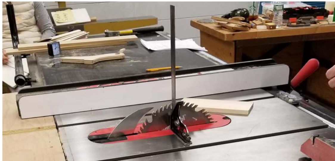
Checking blade's 90 degrees to table
