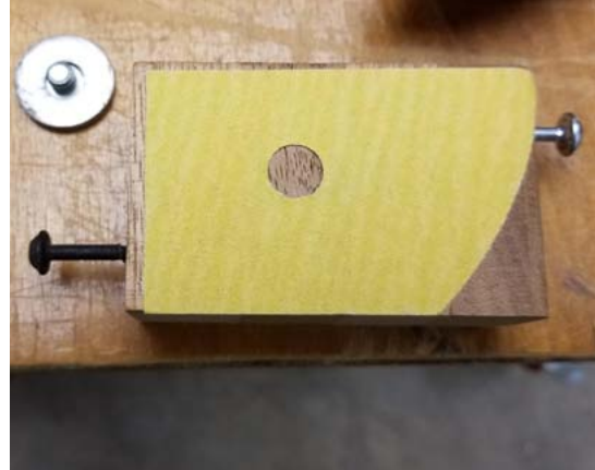
Bob's adjustable block for repeating precise cross cuts
