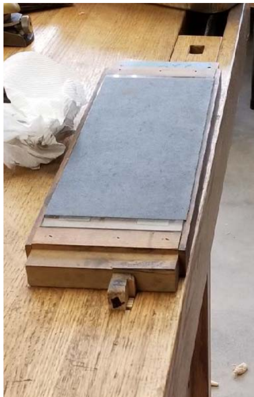
220 wet-dry paper on glass to flatten plane's sole and frog
