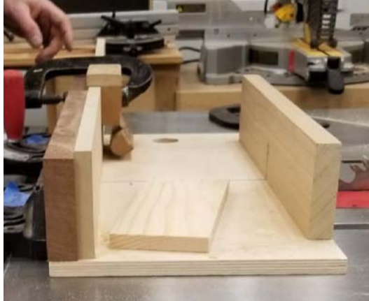
Bob's custom-made sled for cross cuts
