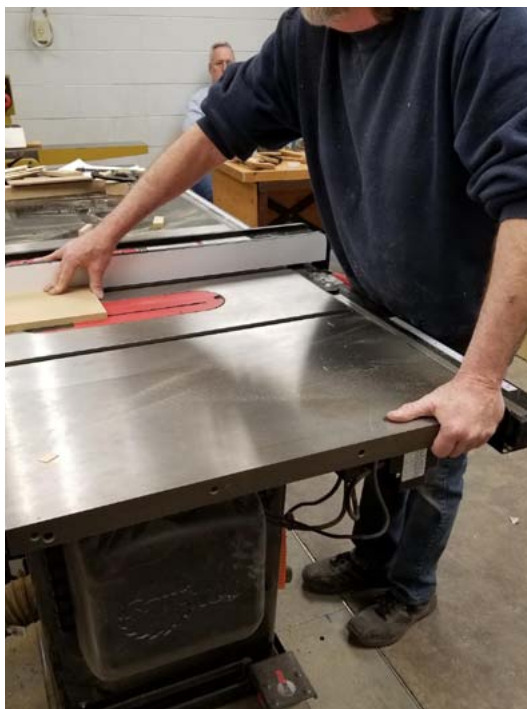
Correct stance and fingers' position for ripping
