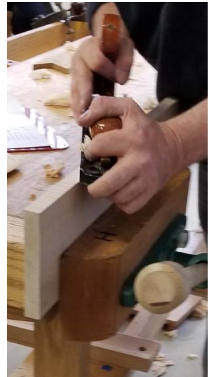
Correct hold while planing with fingers guiding both sides of the board
