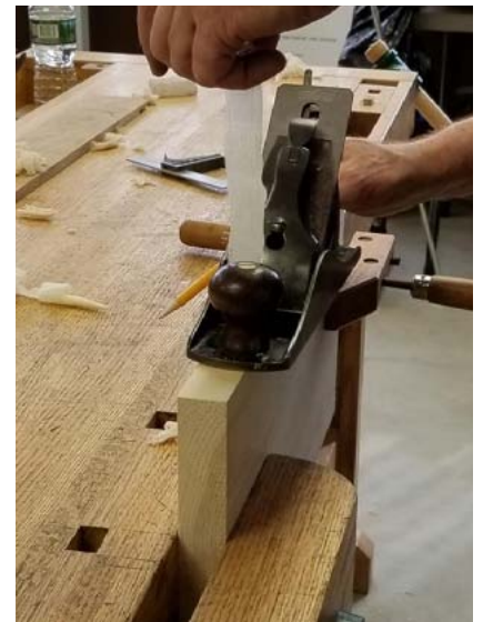
How shavings reveal sharpness and set of a plane
