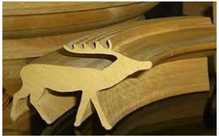
Reifendrehen cross section showing finished ring and design
