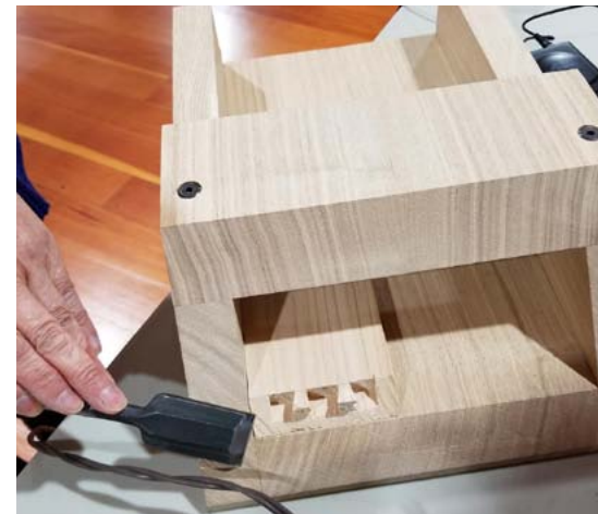
Juliana's jig for mitering dovetails with a chisel
