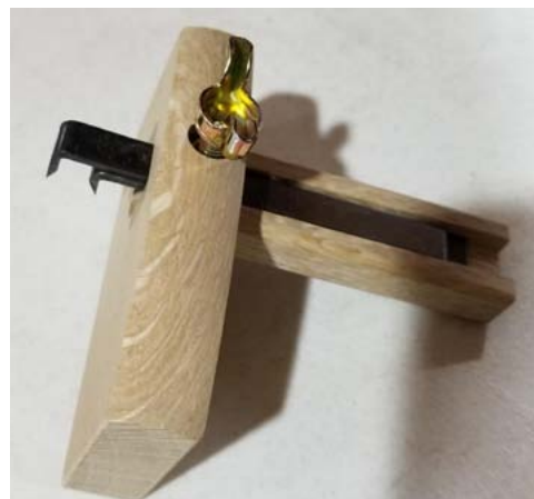
Tenon marking gauge with two blades
