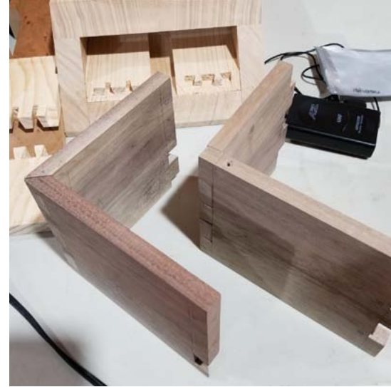
Example of hidden dovetail joints when assembled
