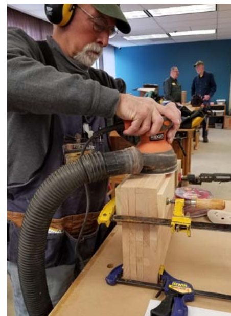
Sanding six boards' edges at a time
