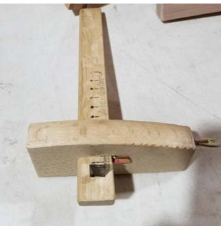
Her marking gauge with etched increments
