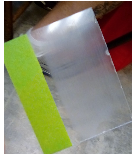
15,000 grit used on acrylic still leaves scratch patterns
