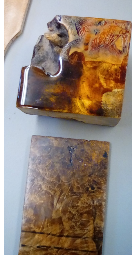
Test surfaces seal-coated with epoxy, cut back and finished
