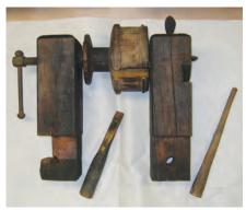
Hurley lathe headstock and pulley assembly
