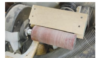
Sanding jig attached to bench grinder
