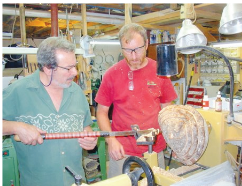
Andy shows Steve Sherman how to define the bowls in the coring process
