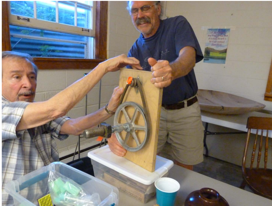
Steve and Ron Roberts display Doug's step down rotisserie for applying urethane. Note that a four jaw chuck can be mounted on the spindle.
