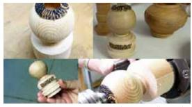
Various texturing treatments used on a small vessel
