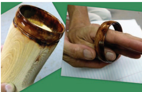
A bangle formed from a cylinder (right) and parted off (left)
