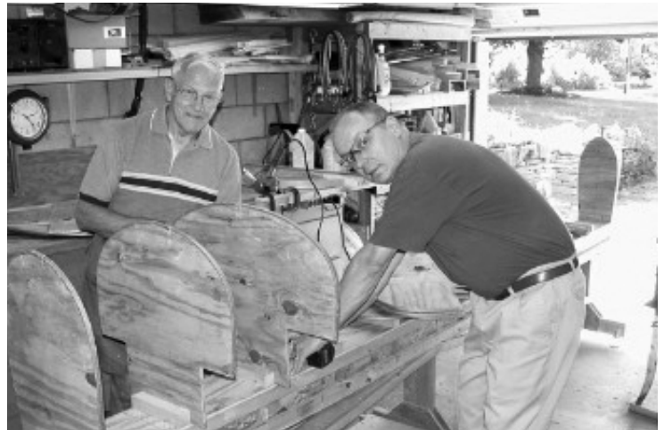
Don Dean and George Walko set up the forms for building a cedar strip canoe.
