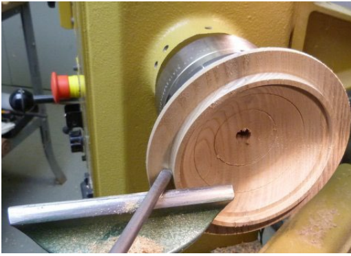
It is critical to ensure the lid tenon is perpendicular
