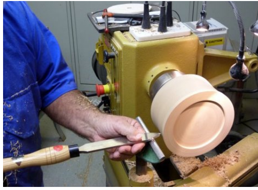
Joe uses a Raffan spear point to start a bead
