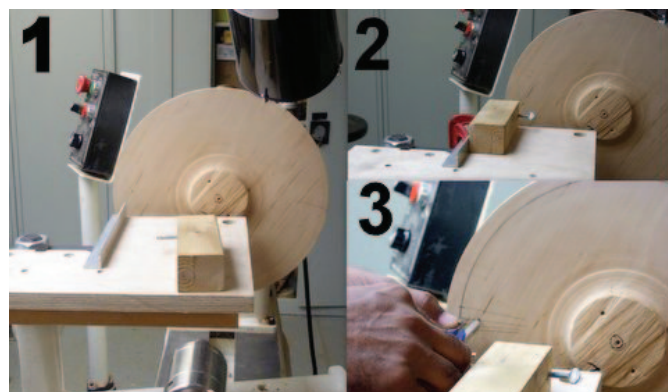
The application of the design depends on 1) a flat stable platform which can hold a pencil at the centerline of the lathe 2) defining a rim line and radius line with a soft pencil and 3) establishing each square in the pattern by setting an equal distance with dividers set to the chosen index spacing.
