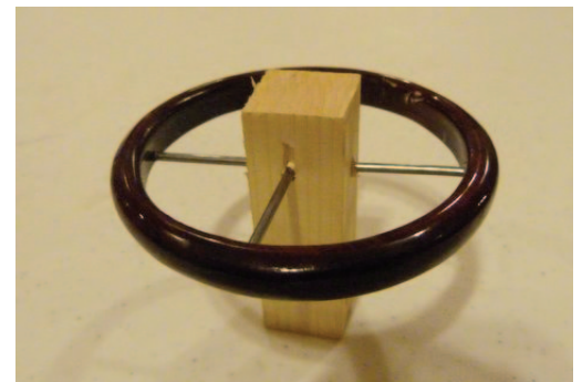
An example of Jim's 'blocks and lightning rods' for holding the bangles during finishing
