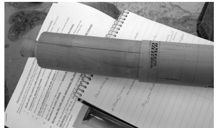
Dowel partially inside turned cylinder - note air groove on dowel
