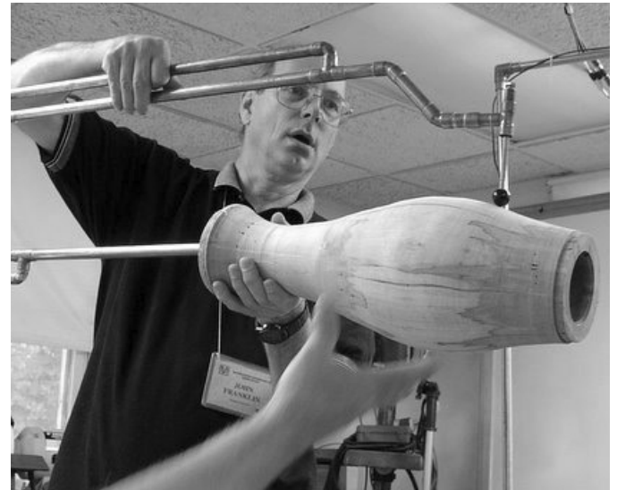
A thickness gauge for deep hollowing
