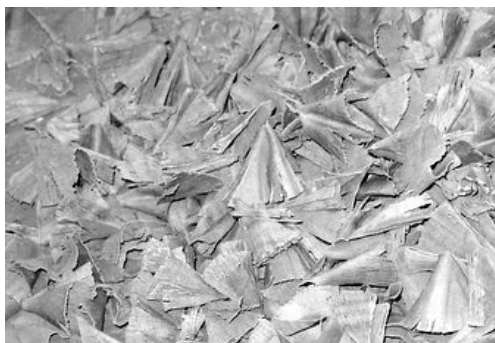
A properly cutting Forstner bit leaves this type of shaving
