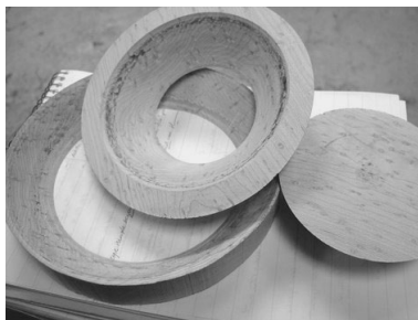
Flat stock with concentric rings parted
