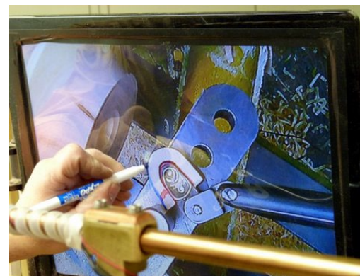
The visualizer approach uses an acetate sheet to mark the dimension of the cutter, as well as the desired thickness. This representation is shown graphically on the screen and moves with the tool.
