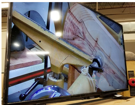
Camera screen demonstration of tenon cut
