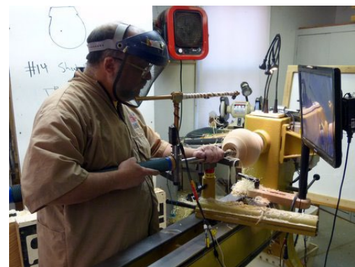
The entire camera and hollowing system in use. Carl concluded that the OEM Bosch Visualizer is the better option than a shop made alternative.
