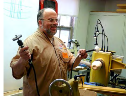
Carl shows the shop made flexible shaft rotary wheel
