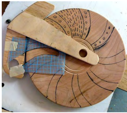
An Al Stirt inspired T Square and acetate sheet used to lay out the design
