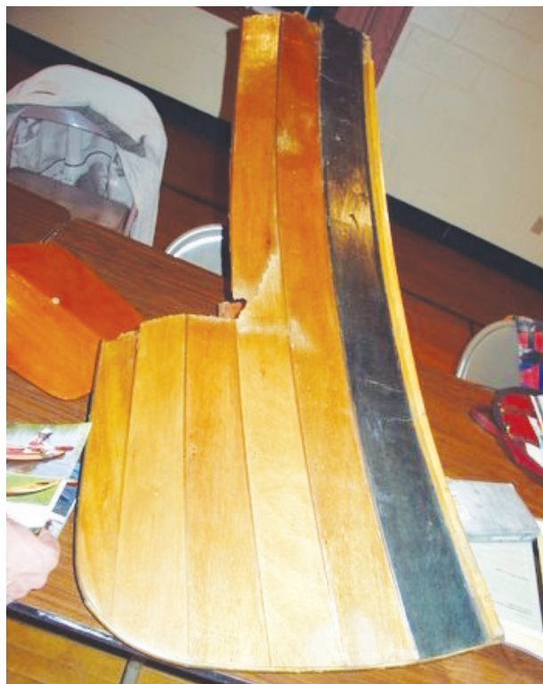
Section of kayak damaged by tree fall -- glue sections held together
