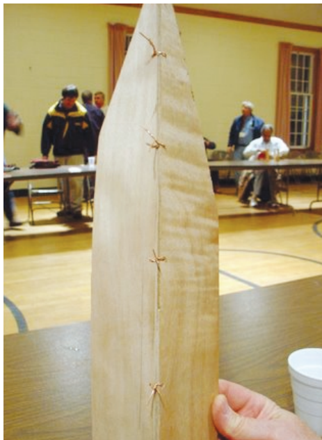
Two boards stitched with copper wire
