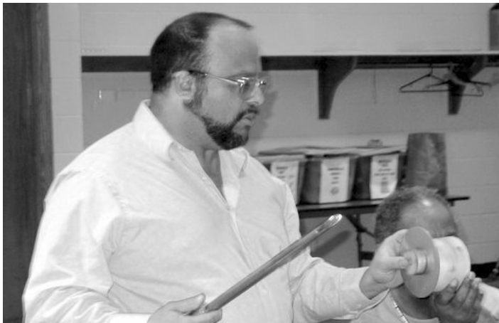
Aluminum disc is pressed over wooden form
