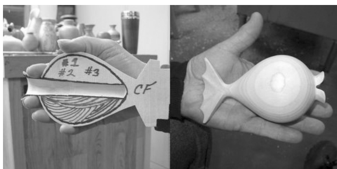
Cutting pattern for the fish form. #1 straight tool, #2 hook tool, #3 straight tool finish bottom
