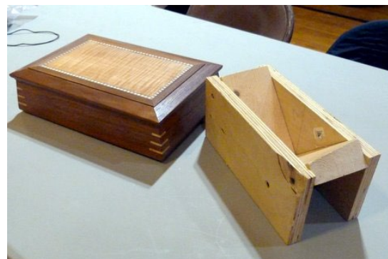
Al Shinker made a sled for spline joints, along with his finished product
