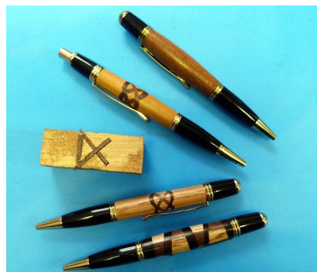
Finished Gatsby pens alongside the rough blank for the Celtic knot
