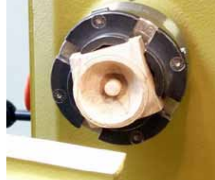
Bill's jam chuck features a ½" dowel as a registration jig for re-chucking the hollow ball
