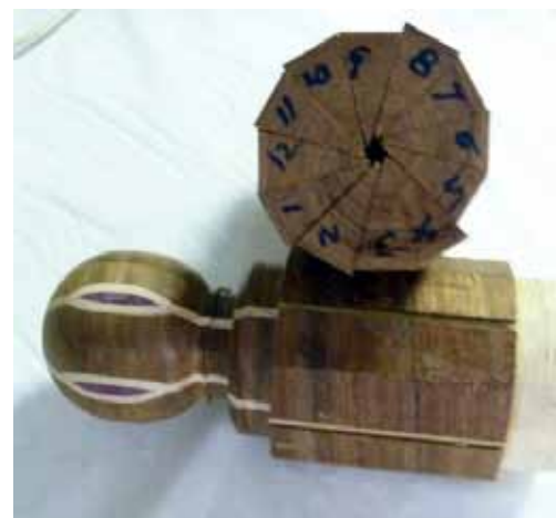
Each stave is numbered to maintain grain direction
