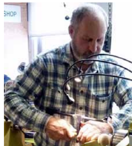
Bill hollows the ball with his modified laser-assisted Nano tool
