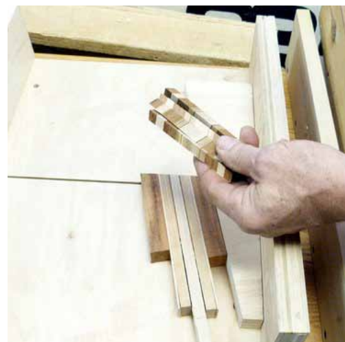
A table saw sled is constructed to ensure 14.8 degree angle cuts to create staves for the ornament
