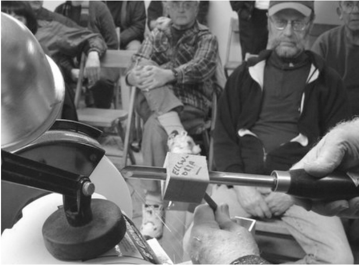
Stan demonstrates jig for performing an Ellsworth grind
