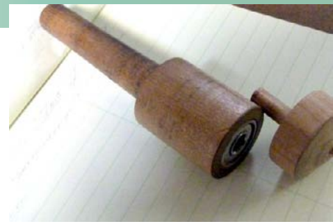
Shop made revolving tailstock that accepts different attachments to hold the delicate ends of finials
