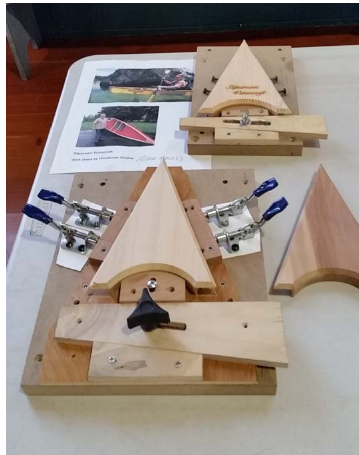
Jig for canoe decks
