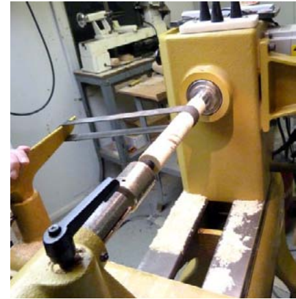
A section of a tire inner tube can act as a brake
