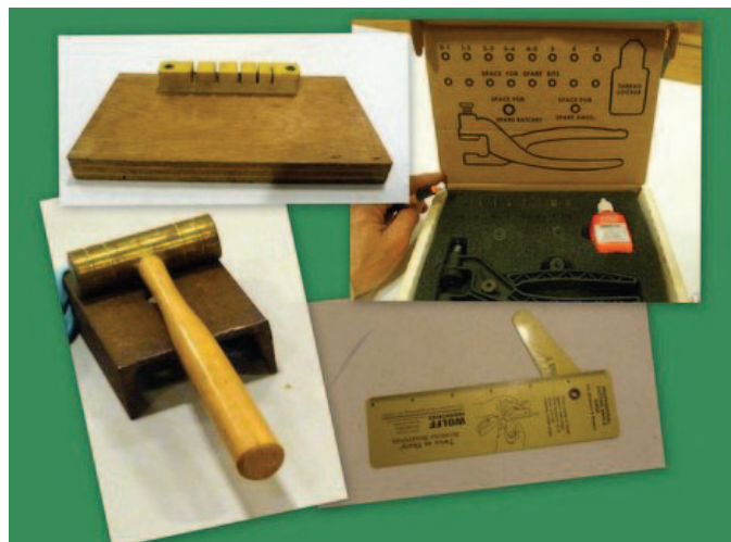
Accessories include holding fixtures for serrated scissors, scissor angle gauge, punch tool for disassembling scissors, and brass hammer for straightening shearing arms
