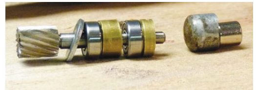
Stacked bearings and spacers awaiting insertion in handle
