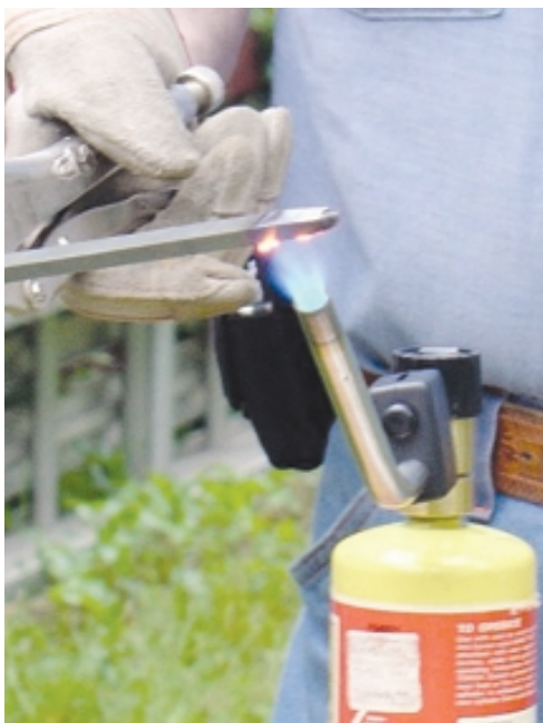
Chuck used MAPP gas to heat the tool stock
