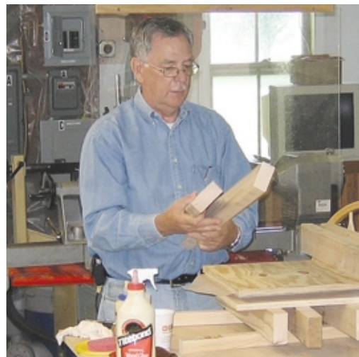
Al Shinker showing cauls and a simple press that uses "F" style clamps.
