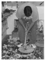
Using an adz to hollow the seat
