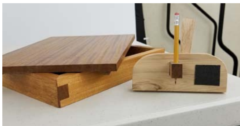
Juliana Shei's hidden dovetail box and marking gauge
