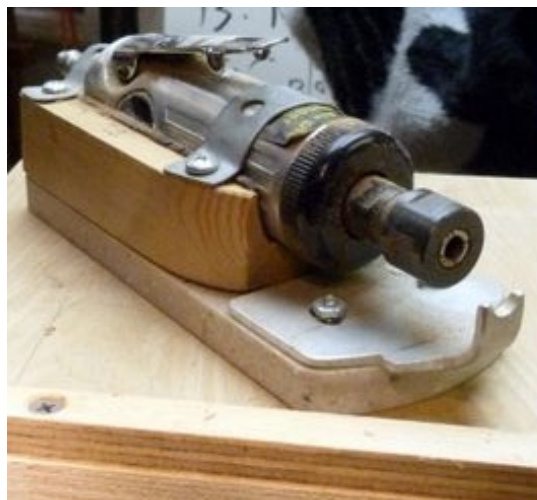
Steve Sherman set up his tilting table, grinder and sled for producing grooves on bowls
