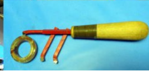
Bill Thiry discusses his shop made tools: top right, mini hollower for ornaments - bottom right, turning tools for cutting marble
