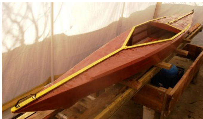
The finished kayak is 14' long and weighs just 23 lbs.
