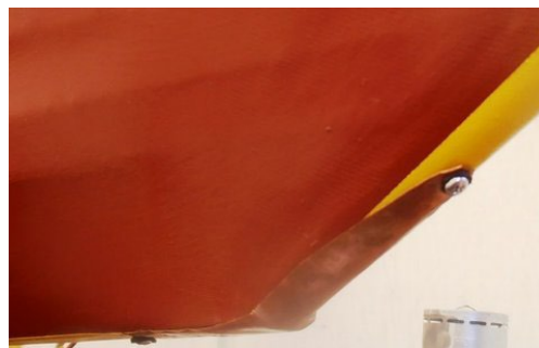
Copper flashing was used as a skid plate
