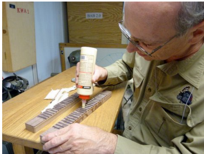
Rip the blank in half and apply glue to the kerf sides, being careful not to get glue the kerfs themselves.
