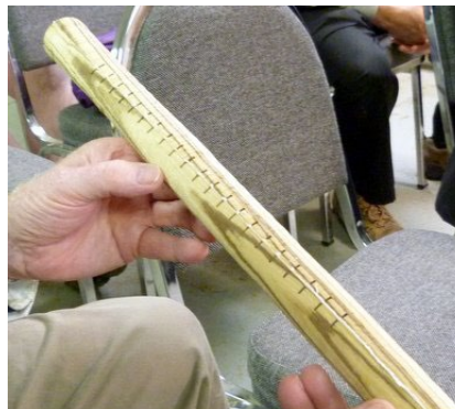
The resultant "sandwich" glue-up is turned into a cylinder. Once carved and finished, the outside kerfs are cut to meet the inside kerfs.
