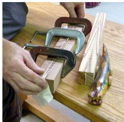
Clamp the pieces together separated by a length of sturdy cloth or other flexible material.
