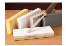
a comparison of the sharpening properties of each and will bring samples of different types of benchstones: aluminum oxide, silicon carbide, Arkansas and waterstones. We will have some sharpening stations set up and you are invited to bring a chisel, plane iron or small knife along so that some of you as time allows can test out the different stones and get a feel for how they perform.
