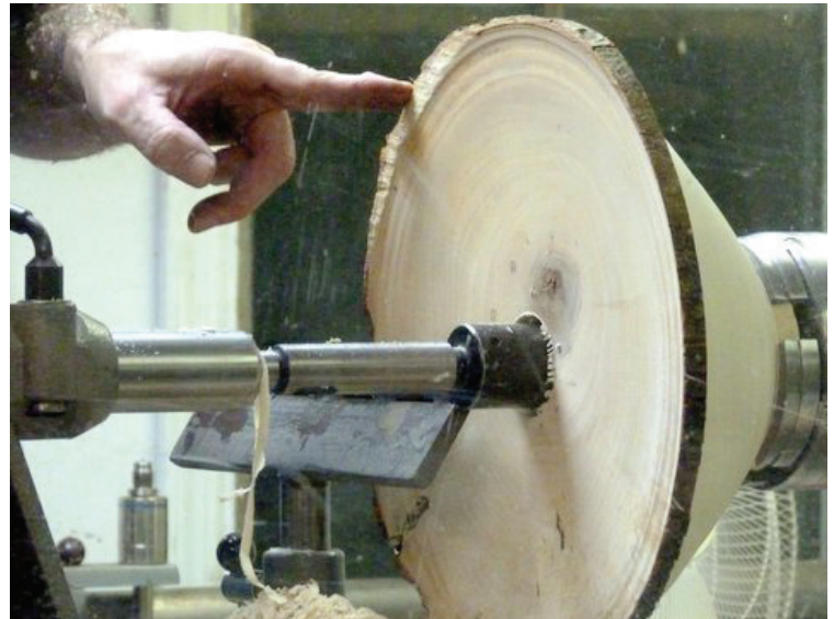
The live center is inserted into a 2" hole in the bowl
