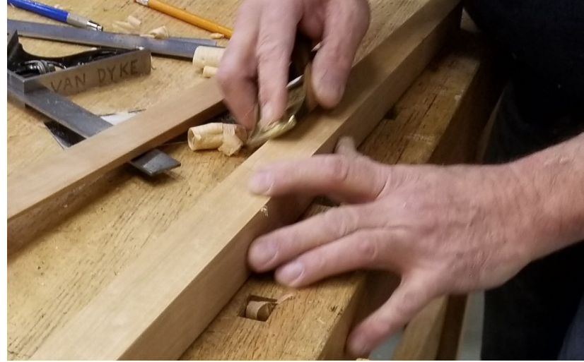
Bob hides the glue line by planing a small bevel on the leg's edge
