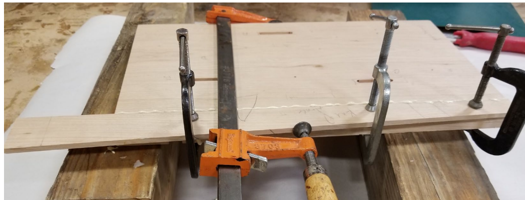
Clamp positions to repair hinge mortise
