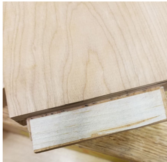
Wood shaving to tighten a tenon
