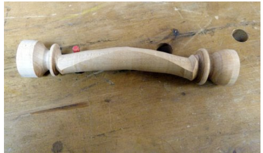
A sample of two axis turning: a combination of coves and beads
