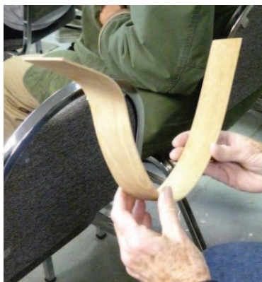
Staves are shaped from two layers of veneer
