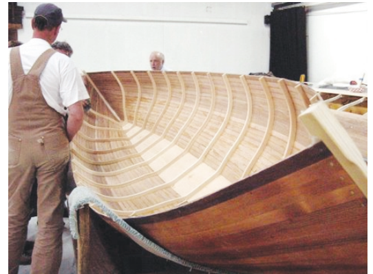
Interior guide boat view showing laminated spruce ribs.
